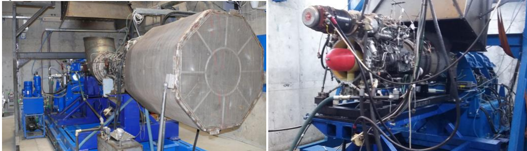
Fig. 5. TV2-117A (left) and TV3-117MT (right) engines into the test bench
