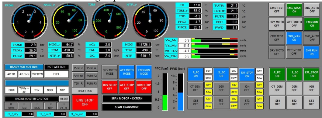
Fig. 4. TV2-117A operator graphic interface
