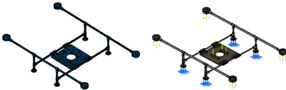
Fig. 2. Finite element frame model with boundary conditions
