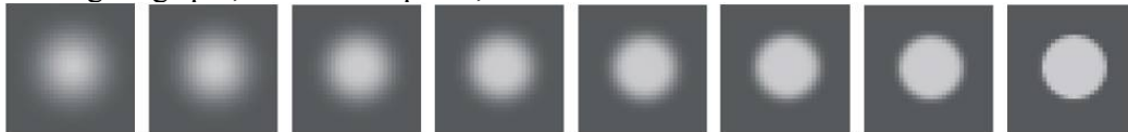
Fig. 9. Pointer spot, acquired on a matrix of 30x30 pixels. Left - defocused, right - focused
