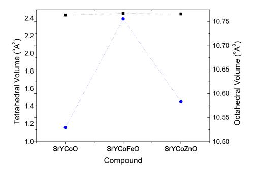
Fig. 4. Volume variations of tetrahedral (black square) and octahedral (blue circle) layer of the three compounds deduced from the refinement results of the associated XRD data.
