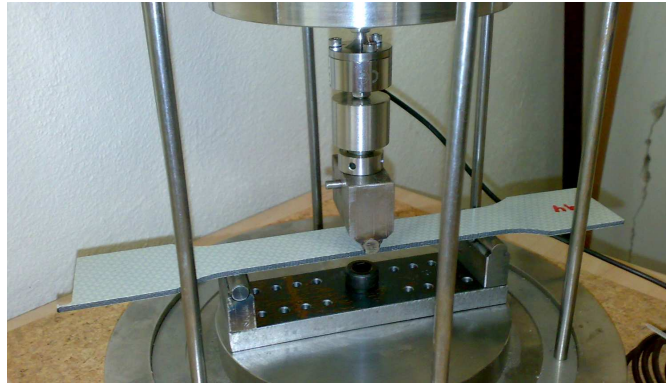
FIGURE 7. Experimental setup for three-point bending. Detail of the grips with load cell in the testing chamber
