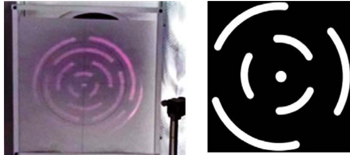
Fig. 4. Mira used for clear evidencing laser beam center
