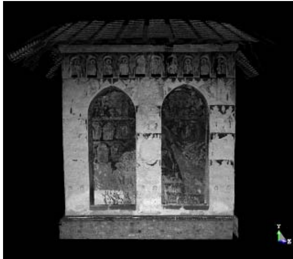
Fig 6 Image containing more than 25 millions of points of the stoop of the Humor church.
