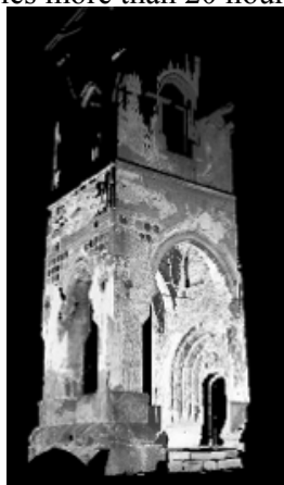
Fig 2 Screen capture of the 3D digital model of the Bălinești stoop, a model represented by 56millions of points at a medium resolution of 1.5 mm
