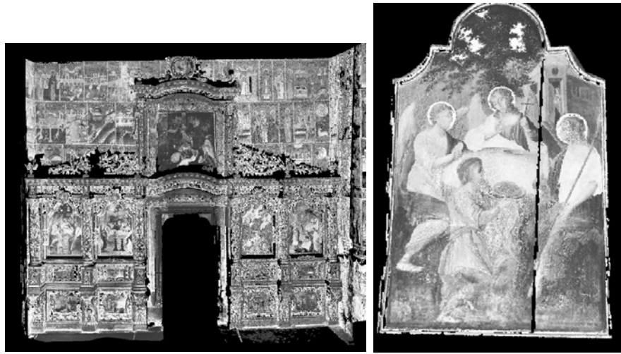
Fig. 4 The iconostas of the Sucevița church reconstructed by more than 20 millions of points, at a medium resolution of 0.8mm with 5 scans. On the left side of Sucevița's iconostas was a cutting on one of the icons. The distance between the slices varies from 0.3 up to 1.6 mm, image containing 1 millions of points.
