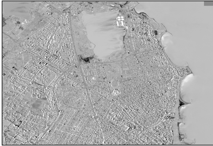
Fig. 7. Changes between 2000-2005 on Northern part of Constantza town on PCA analysis for images Landsat ETM7+ 12/08/2000 images and Landsat ETM7+ 24/08/2005 (dark areas represent changes)
